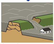
The water then starts to escape through the cracks in the levee.
